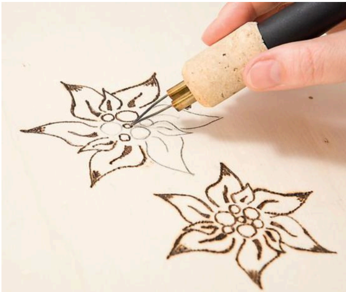
Step 1) Trace contours with the fine tip of the firing station.
